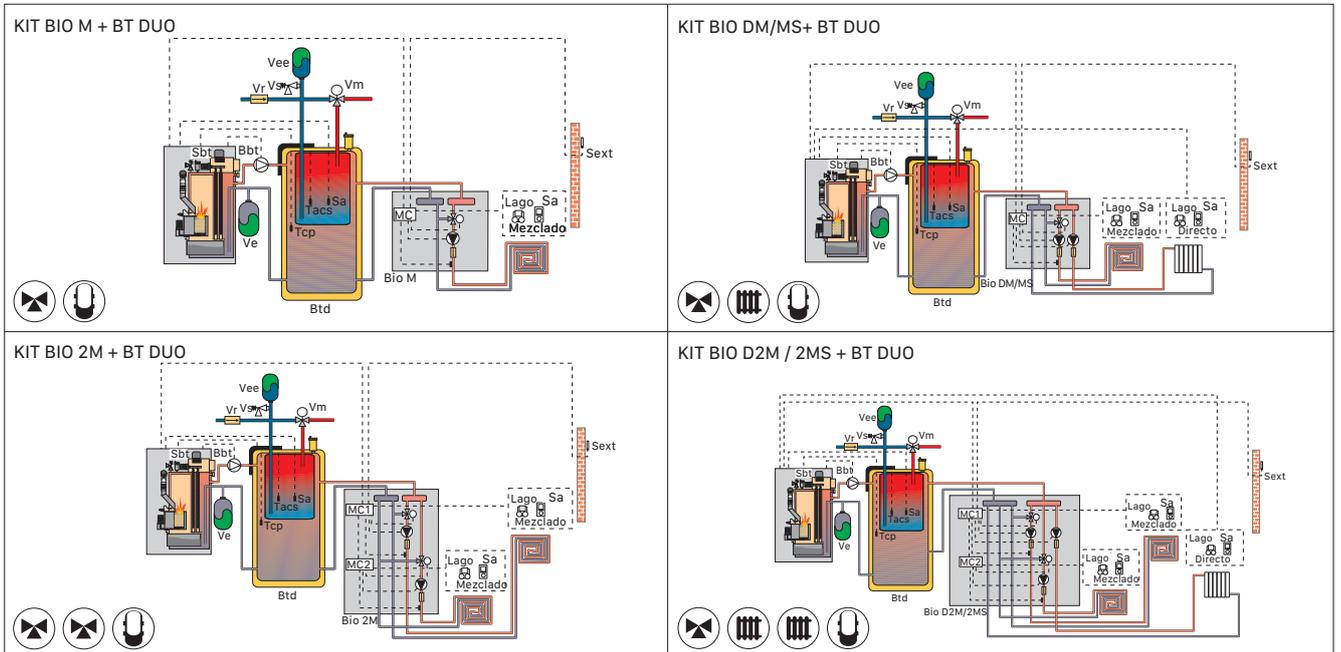
**KITS HIDRÁULICOS CON COLECTOR (IDA Y RETORNO) Y DEPÓSITO DE INERCIA BT DUO**
