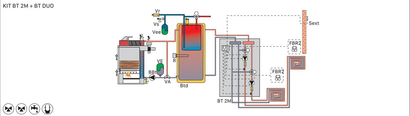
**KITS HIDRÁULICOS CON COLECTOR (IDA Y RETORNO) + DEPÓSITO DE INERCIA BT**
